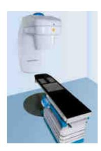
Bhabhatron, the radiotherapy device developed by BARC, revolutionised cancer treatment in the country by providing an affordable, high-performance Co-60 teletherapy machine
